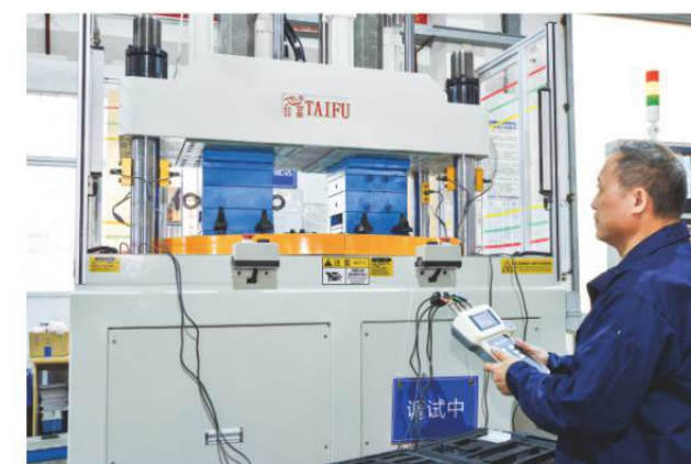
哥林柱检测 Tiebar detection
